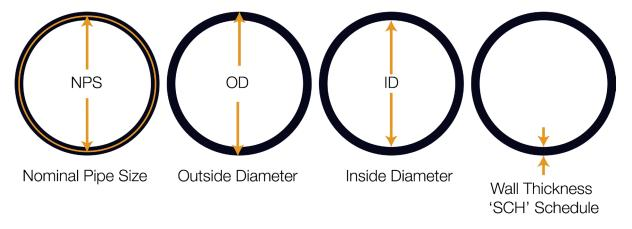
Nominal Pipe Size (NPS) originates from a North American set of standard sizes for pipes with the commonly used terminology of eg 2 inch, 4 inch, 6 inch etc having a historical association with the time when 'inch' referenced the actual ID.
