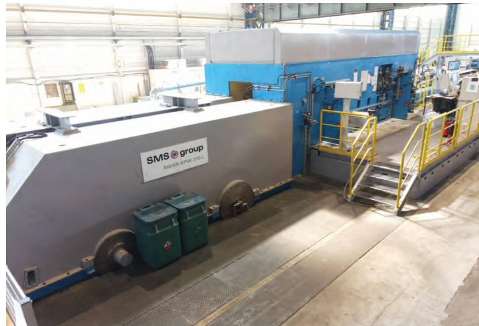
The newly commissioned KP2 at MST’s Remscheid plant is the world’s largest cold pilgering machine.
